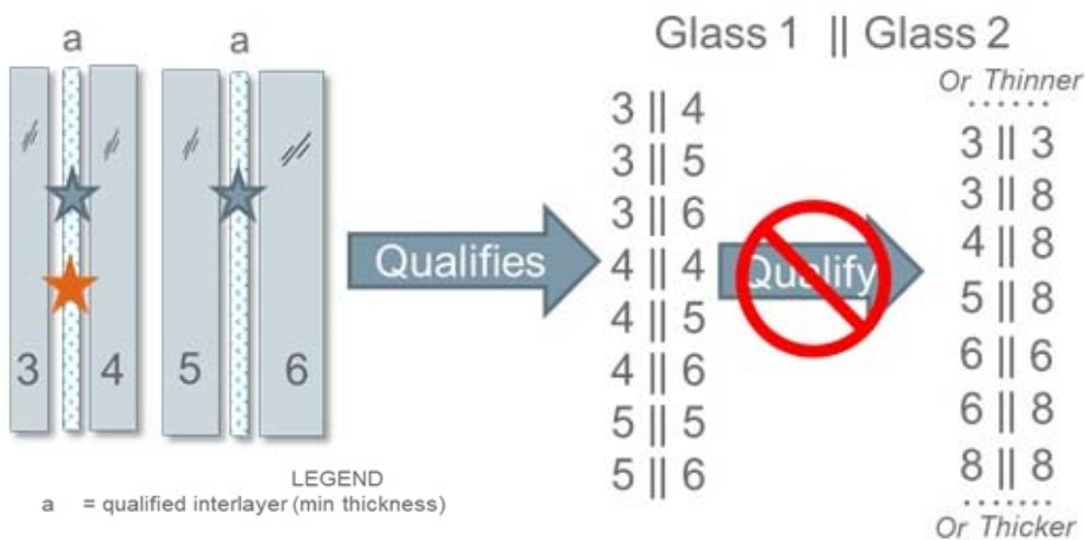
Figure 2 – Example of initial and ongoing laminated glass thickness submission with asymmetrical glasses
